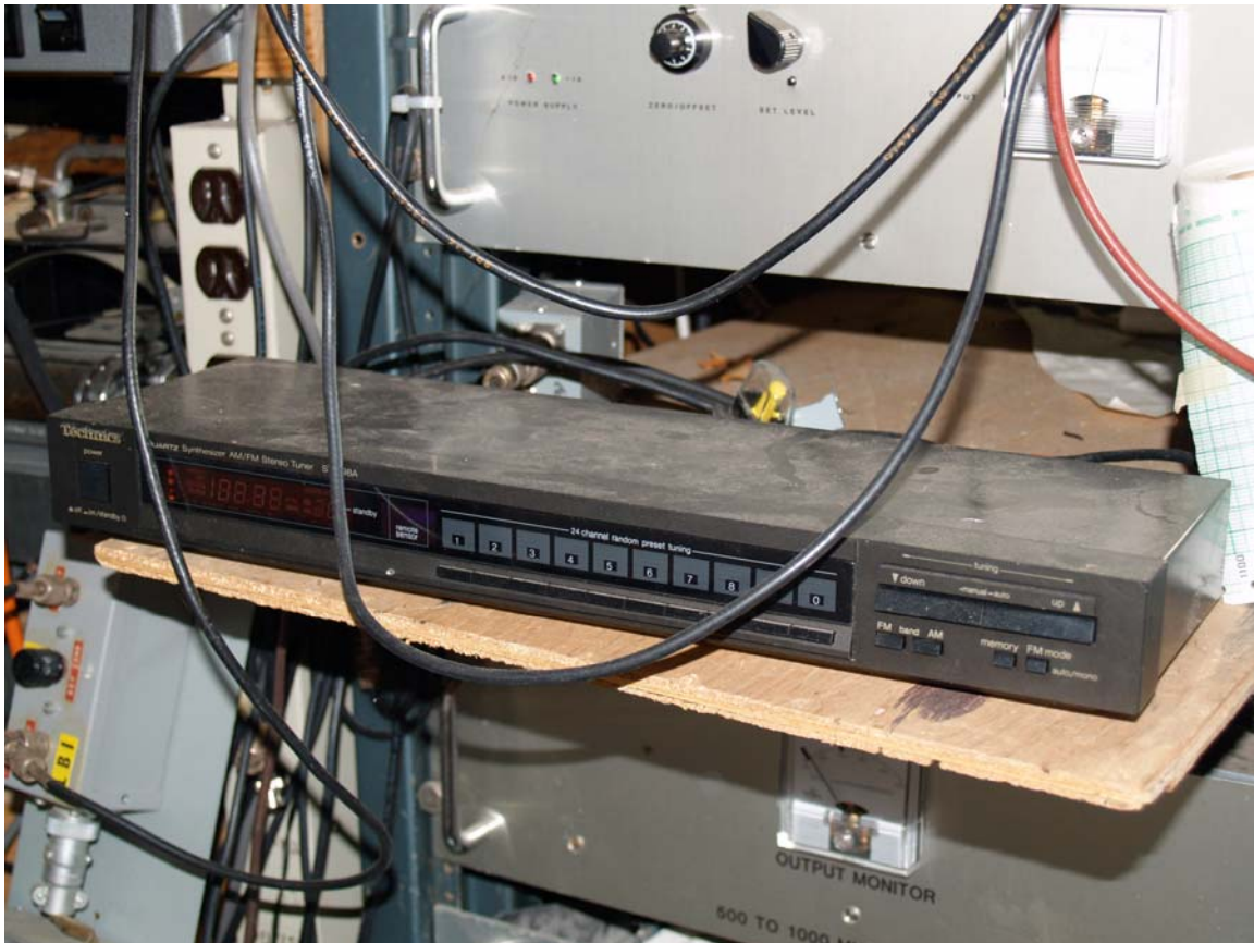
Figure 2: The meteor receiver is an old FM tuner, with access to the LO Lock light to detect meteor signals. The silver box above contains a DC amplifier and computer interface.
