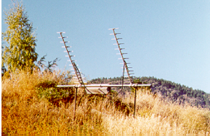
Figure 1: The eastern end of the interferometer. The signals from the two yagis are combined in a 2:1 combiner. The box attached to the elevation axis contains a filter and the first GaAsFET amplifier. Mounting the yagis so that the axis is behind the reflector elements reduces the interaction between the antennas and mount.
